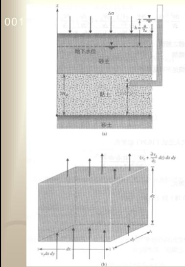
$$\frac{\partial \bar{u}}{\partial t} = c_v \frac{\partial^2 \bar{u}}{\partial z^2}$$
