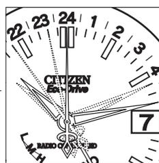
◆ When the reception is successful, the second hand will return to 1-second interval movement and the other hands will be automatically corrected.
