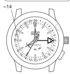
After setting the time, return the crown to its normal position; the second hand will move normally, and the 24-hour hand will display the set time.
