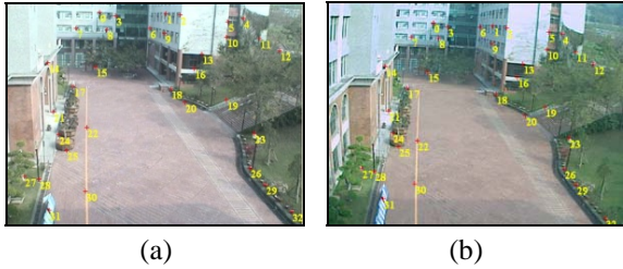
Figure 5. An example of false match elimination: (a) the image of the wide-angle camera, (b) the image of the PTZ camera
