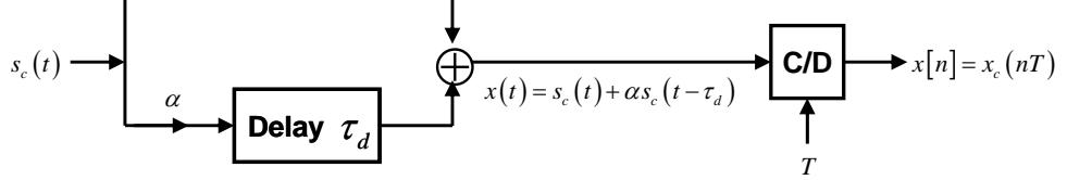
$$X_c(j\Omega) = \Im\{s_c(t) + \alpha s_c(t - \tau_d)\} = S_c(j\Omega)(1 + \alpha e^{-j\Omega\tau_d}).$$
