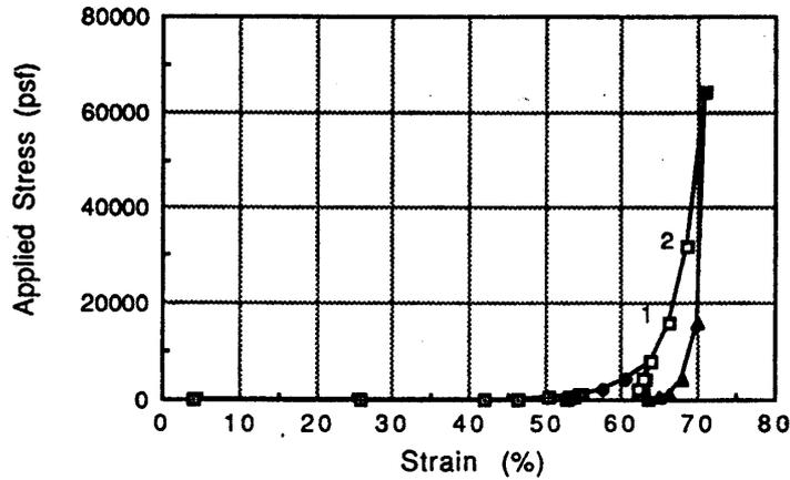
Fig. 1.1a Stress-Strain Curve for One-Dimensional Compression of Soft Clay
