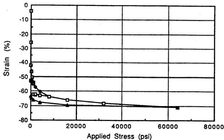
Fig. 1.1b Rotated Stress-Strain Curve for Soft Clay in One-Dimensional Compression
