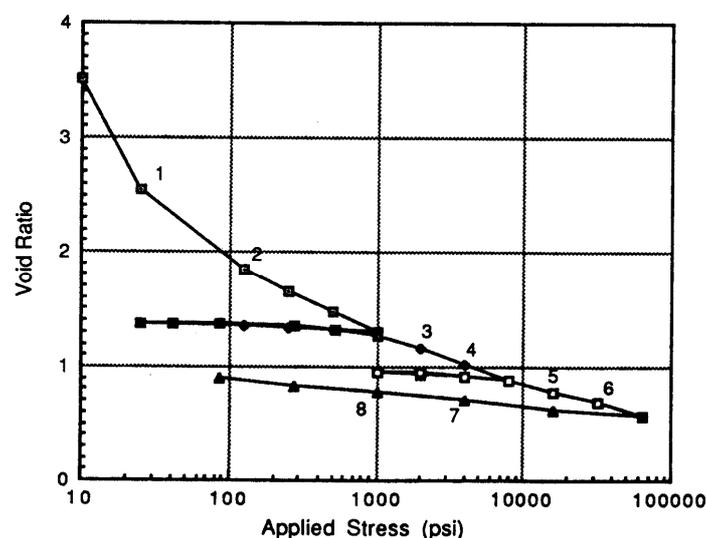
Fig. 1.1d Stress-Strain Curve for Soft Clay, Plotted using Logarithmic Stress Axis and Void Ratio for Strain
