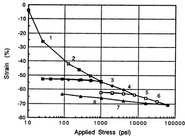
Fig. 1.1c Semi-Logarithmic Plot of Stress-Strain Curve Used to Provide More Detail at Small Stresses
