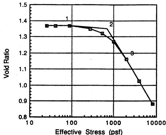
Fig. 1.2 Use of Bilinear Stress-Strain Curve to Approximate Actual Curve
