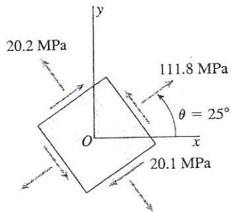
$$\begin{aligned}\sigma_x &= 80 \text{ MPa} & \sigma_y &= 52 \text{ MPa} & \tau_{xy} &= 48 \text{ MPa} \\ \theta &= 25^\circ \\ \sigma_{x_1} &= \frac{\sigma_x + \sigma_y}{2} + \frac{\sigma_x - \sigma_y}{2} \cos 2\theta + \tau_{xy} \sin 2\theta \\ &= 111.8 \text{ MPa} \\ \tau_{x_1y_1} &= -\frac{\sigma_x - \sigma_y}{2} \sin 2\theta + \tau_{xy} \cos 2\theta \\ &= 20.1 \text{ MPa} \\ \sigma_{y_1} &= \sigma_x + \sigma_y - \sigma_{x_1} = 20.2 \text{ MPa}\end{aligned}$$
